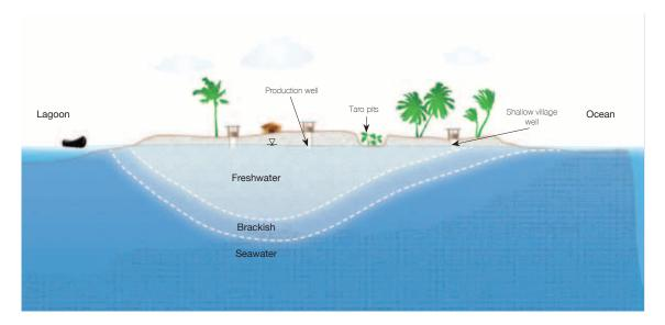
Figure 2.5: Concept model of atoll groundwater.
